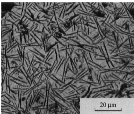
Fig. 2. Optical micrograph of the as-cast  $Mg_{65}Cu_{20}Zn_5Y_9Zr_1$  composite.
