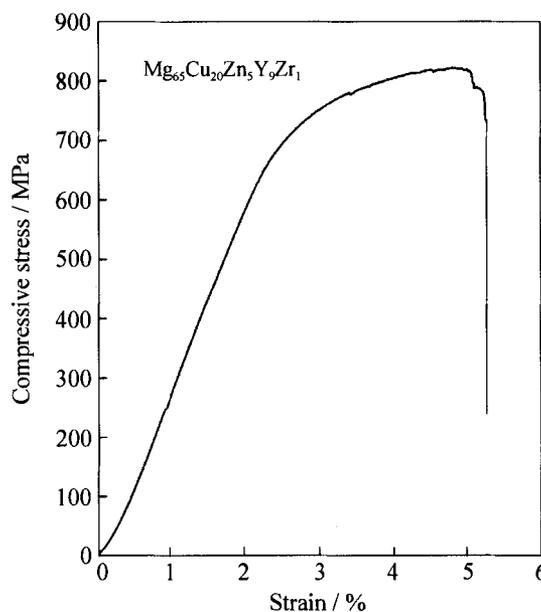
Fig. 4. Compressive stress-strain curve of the bulk  $Mg_{65}Cu_{20}Zn_5Y_9Zr_1$  composite with a diameter of 2 mm.
