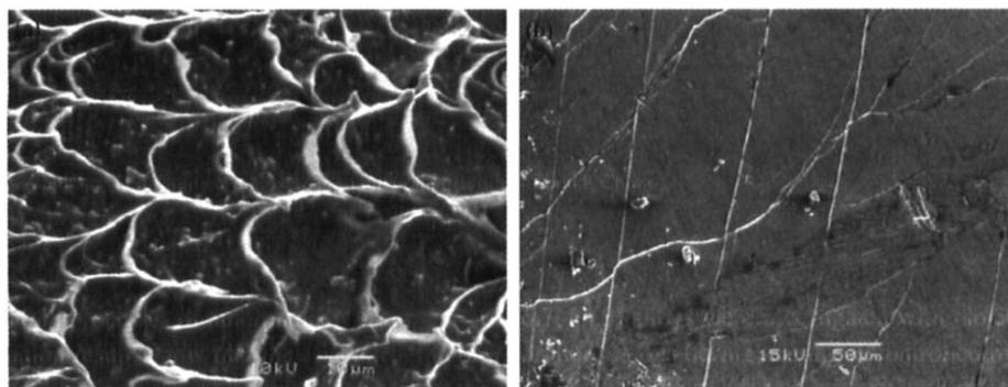
Fig. 5. SEM images of the surface morphology of the fractured  $Mg_{65}Cu_{20}Zn_5Y_9Zr_1$  composite: (a) the fracture surface; (b) the lateral surface.
