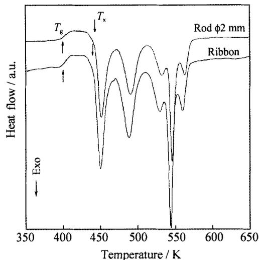
Fig. 3. DSC curves of the  $Mg_{65}Cu_{20}Zn_5Y_9Zr_1$  alloy ribbon and cast rod with a diameter of 2 mm.
