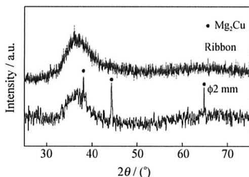
Fig. 1. XRD patterns of the  $Mg_{65}Cu_{20}Zn_5Y_9Zr_1$  alloy ribbon and cast rod with a diameter of 2 mm.
