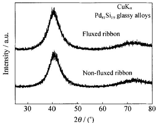
Fig. 1. XRD spectra of Pd<sub>81</sub>Si<sub>19</sub> glassy alloys.
