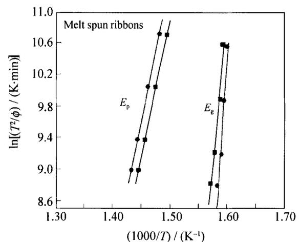
Fig. 3. Kissinger curves of crystallization of the fluxed Pd<sub>81</sub>Si<sub>19</sub> ribbons marked with circle and the non-fluxed ones marked with square.
