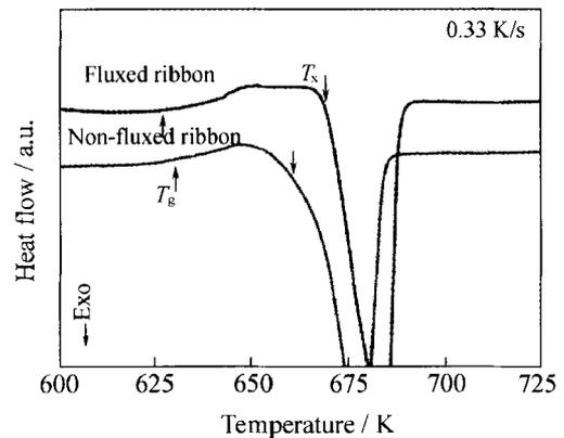
Fig. 2. DSC curves of both fluxed and non-fluxed Pd<sub>81</sub>Si<sub>19</sub> glassy ribbons.
