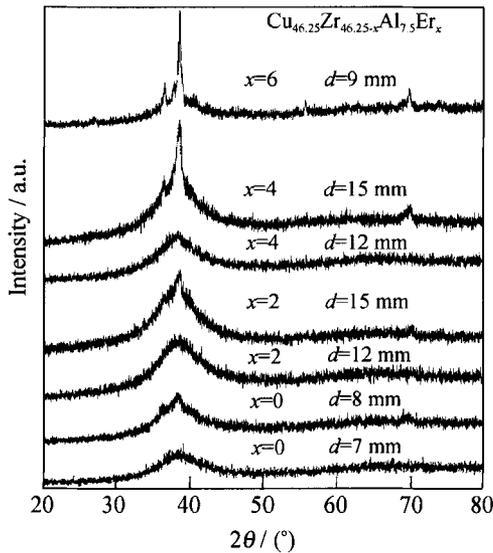
Fig. 1. XRD patterns of  $\text{Cu}_{46.25}\text{Zr}_{46.25-x}\text{Al}_{7.5}\text{Er}_x$  ( $x=0, 2, 4,$  and  $6$ ) alloy rods with various diameters ( $d$  denotes the diameters of rods).
