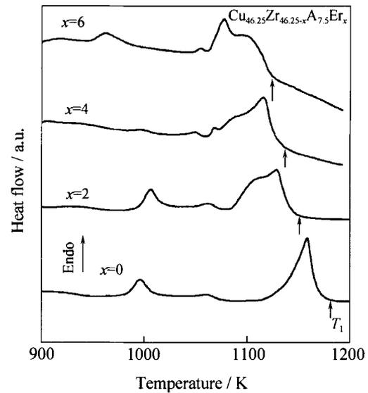
Fig. 4. Melting behaviors of  $\text{Cu}_{46.25}\text{Zr}_{46.25-x}\text{Al}_{7.5}\text{Er}_x$  ( $x=0, 2, 4, \text{ and } 6$ ) alloys at a heating rate of 0.333 K/s.
