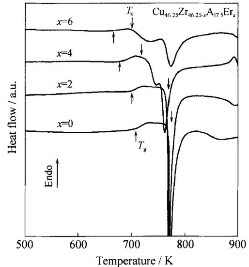
Fig. 3. DSC curves of melt-spun  $\text{Cu}_{46.25}\text{Zr}_{46.25-x}\text{Al}_{7.5}\text{Er}_x$  ( $x=0, 2, 4$  and  $6$ ) glassy ribbons at a heating rate of  $0.333$  K/s.
