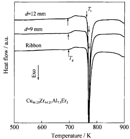
Fig. 2. DSC curves of as-quenched ribbon and as-cast rods with  $d=9$  and  $12$  mm for  $\text{Cu}_{46.25}\text{Zr}_{44.25}\text{Al}_{7.5}\text{Er}_2$  alloy.
