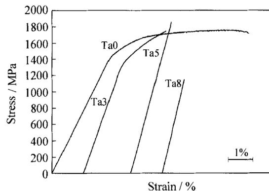
Fig. 5. Compressive stress-strain curves at room temperature for  $(\text{Ti}_{0.4}\text{Zr}_{0.25}\text{Ni}_{0.08}\text{Cu}_{0.09}\text{Be}_{0.18})_{100-x}\text{Ta}_x$  ( $x=0, 3, 5, 8$ ) alloys.
