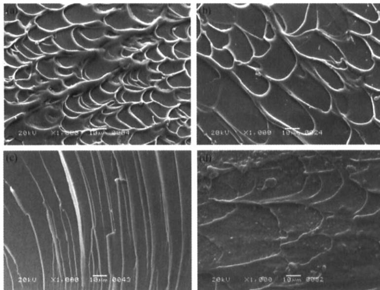
Fig. 6. SEMs of the fracture surface of the failed  $(\text{Ti}_{0.4}\text{Zr}_{0.25}\text{Ni}_{0.08}\text{Cu}_{0.09}\text{Be}_{0.18})_{100-x}\text{Ta}_x$  ( $x=0, 3, 5, 8$ ) alloys: (a) Ta0; (b) Ta3; (c) Ta5; (d) Ta8.
