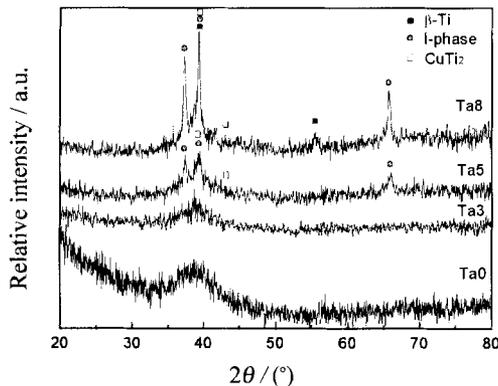
Fig. 1. XRD patterns obtained from  $(\text{Ti}_{0.4}\text{Zr}_{0.25}\text{Ni}_{0.08}\text{Cu}_{0.09}\text{Be}_{0.18})_{100-x}\text{Ta}_x$  ( $x=0, 3, 5,$  and  $8$ ) alloys.
