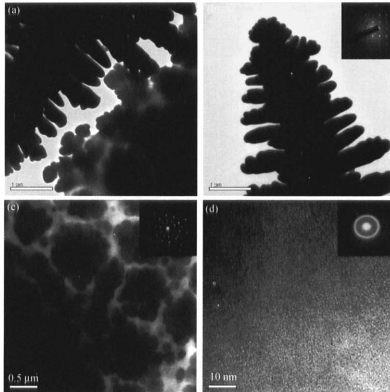
Fig. 3. Typical bright field image obtained from amorphous/quasicrystalline/dendritic structure in Ta8 alloy (a), dendrite (b), quasicrystal (c), and amorphous matrix (d).
