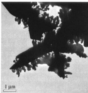
Fig. 4. Typical bright field image obtained from  $\text{CuTi}_2$  phase in Ta8 alloy.
