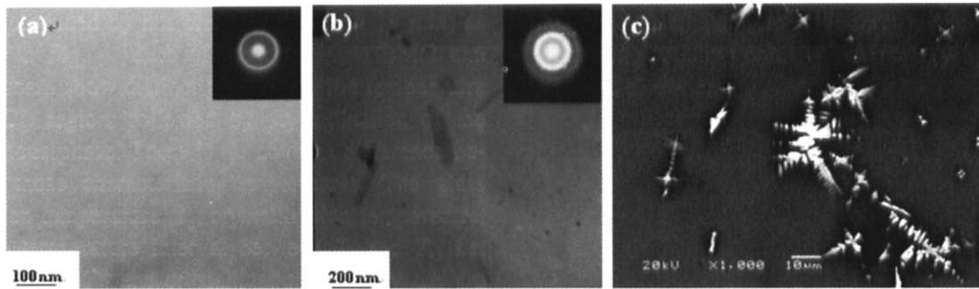
Fig. 2. Microstructure of as-cast  $(\text{Ti}_{0.4}\text{Zr}_{0.25}\text{Ni}_{0.08}\text{Cu}_{0.09}\text{Be}_{0.18})_{100-x}\text{Ta}_x$  ( $x=3, 5, 8$ ) alloys: TEM images of Ta3 (a) and Ta5 (b); SEM image of Ta8 (c).
