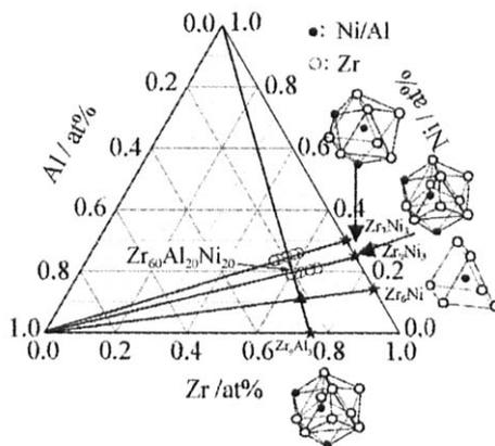
Fig. 2. Composition chart of the Zr-Al-Ni system. Clusters and cluster lines are listed open circles represent bulk metallic glass compositions.
