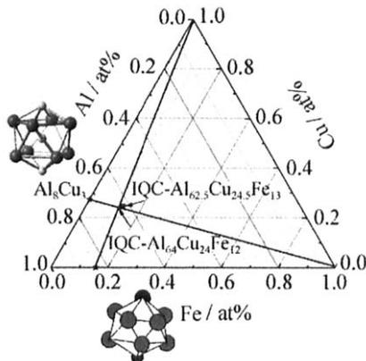
Fig. 1. Schematic composition chart of Al-Cu-Fe. Icosahedral quasicrystal (IQC) is related to icosahedron  $\text{Al}_{10.7}\text{Fe}_2$  and capped Archimedes anti-prism  $\text{Al}_8\text{Cu}_3$ .
