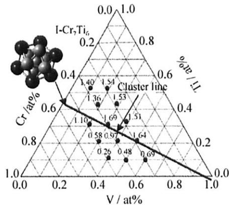
**Fig. 3.** Composition chart of the Ti-Cr-V ternary system. The cluster line  $\text{Cr}_7\text{Ti}_6\text{-V}$  is plotted and the Hydrogen storage capacities of Ti-Cr-V alloys at 303 K [13] are listed.
